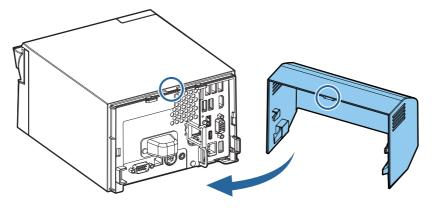
**2** Push the connector cover to click onto the main body.
