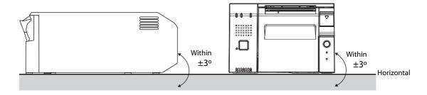
If the printer installation does not fit within the specifications shown in the figure below, the following problems may occur.
