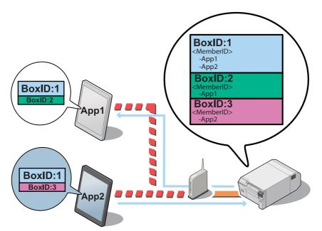
The TM-DT software manages the communication box with a box ID (BoxID in the figure above). Data can be exchanged between applications that belong to the communication box.
