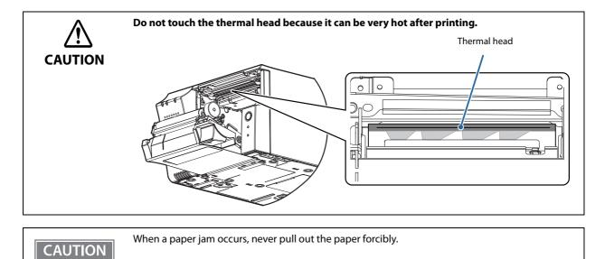
When paper is jammed, never pull out the paper forcibly. Open the roll paper cover"Installing and Replacing Roll Paper" on page 110, and then remove the jammed paper.
