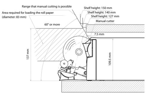
When you install the printer in an enclosed area such as a shelf, secure the following space between the printer and the shelf to avoid heat staying inside.
