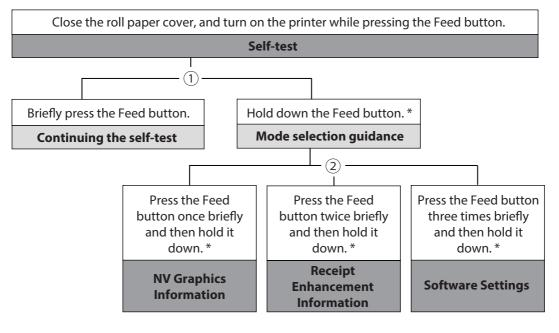
Open the roll paper cover, and turn on the printer while pressing the Feed button, and then close the roll paper cover.
