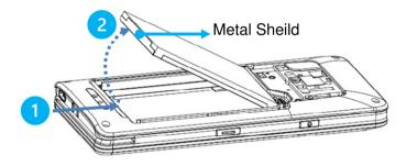
Disconnect the battery by pulling the Molex connector upwards.
