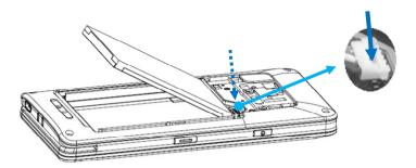
• Insert the battery into the compartment.
