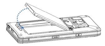
• Place the battery cover and snap into place to secure.
