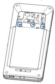
• Place the access point cover and snap into place to secure.
