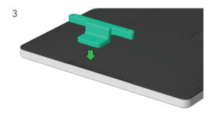
Gently insert the fingerprint reader into the peripheral bay taking care to ensure the connector mates properly.
