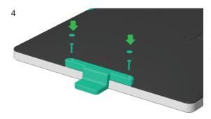
Install the 2 flat head screws included with the kit and cover the screws with the adhesive mylar covers if desired.
