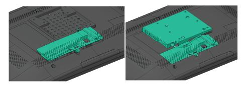
3. Assemble bracket to display. Use screws from bag A for 15.6" display. Use screws from bag B for 21.5" display.
