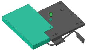
2. Remove I/O door from I-Series. Plug hub USB-C cable into I-series. Reinstall I/O door.
