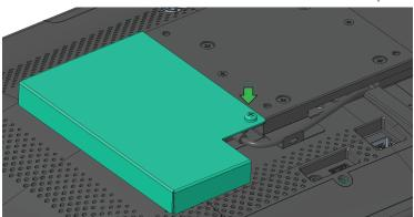
5. Install cable tie from bag D through hole in bracket to secure cables. Assemble stand (not included) using screws from bag C.
