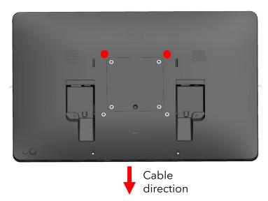
Add (2) screws from bag "L" to top 100 mm VESA positions. Leave ~3mm (1/8") gap for mounting to display bracket. Remove cable cover(s) before mounting displays on stand. See Wallaby<sup>™</sup> assembly instructions (QIG600073 steps 1-5 for counter stand, or QIG600074 steps 1-7 for floor stand) before proceeding.
