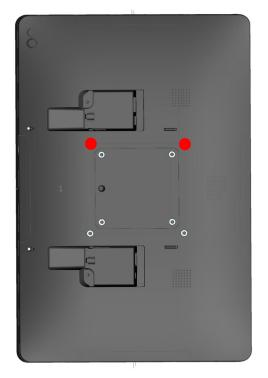
Add (2) screws from bag "L" to top 100mm VESA positions. Leave ~3mm (1/8") gap for mounting to display bracket. Remove cable cover(s) before mounting displays on stand. 2
