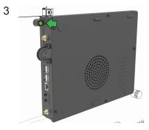
Use a screw driver to tighten the ECM security screw. The security screw must be installed to ensure the ECM does not come out inadvertantly.
