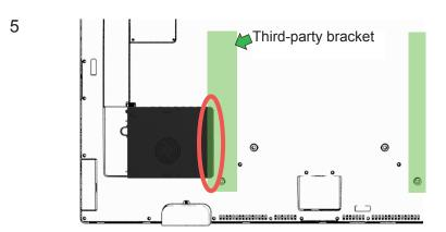
Some third-party VESA mounting systems may interfere with installation or removal of the ECM. The ECM kit includes a set of 15mm spacers and longer mounting screws to add additional clearance between the VESA mount and the ECM. Do not block any air venting on the ECM or IDS display.
