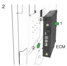
Place the ECM guide rails over the corresponding guides on the rear of the IDS Display and then slide it back toward the docking connectors. Visually inspect it to make sure it seated completely.
