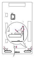
3 Then connect the speaker cable. After installing your speakers, organize the speaker cables.
